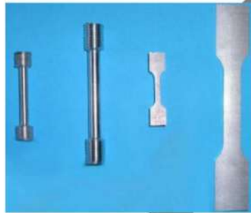
Figure 2-12: Smooth Tensile specimen shapes ( https://it.m.wikipedia.org/wiki/File:Tensile_specimen-round_and_flat.jpg )
