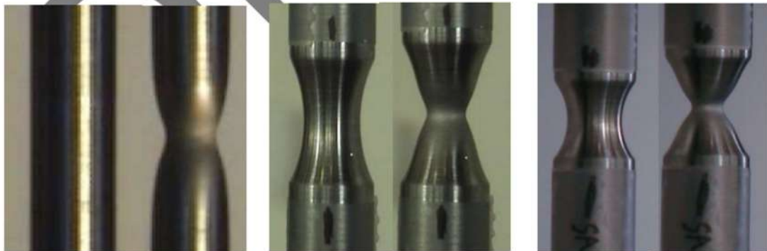
Figure 3-11 Necked specimens with and without notches: initial and necked shapes
