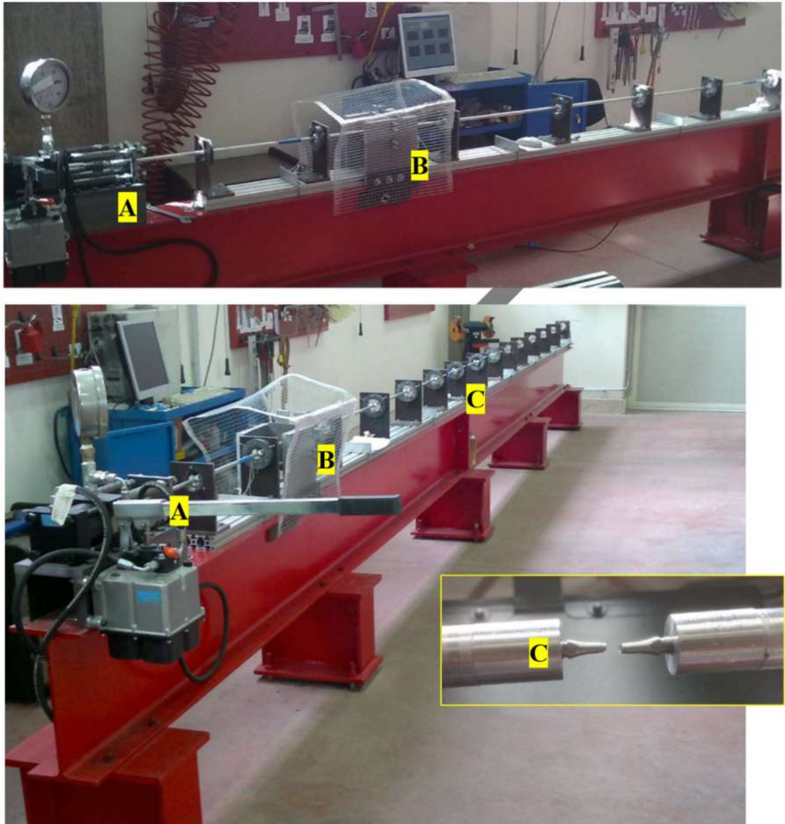
Figure 7-1 Overall view of the Hopkinson bar equipment available at the Mechanics Laboratory of the University of Catania
