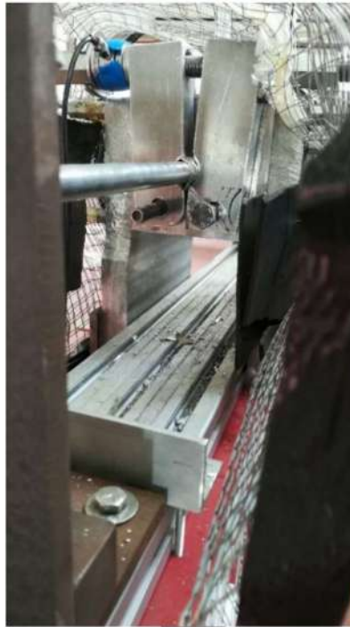
Figure 7-8 Clamping system tightened at end of test preparation: further tightening ruptures the fragile element and starts the test
