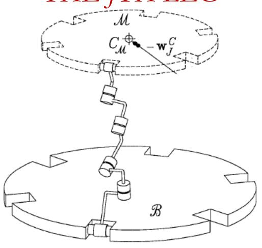
The moving platform  $\mathcal{M}$  has been replaced by the constraint wrench transmitted by the moving platform onto the end link of the Jth leg,  $-\mathbf{w}_J^{\mathcal{C}}$ , whose sign is the opposite of that transmitted by this leg onto  $\mathcal{M}$  by virtue of Newton's third law. The dynamics model of the manipulator then takes the form:
