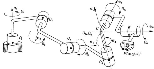
**Decoupled manipolators** are those whose last three joints have intersecting axes.
