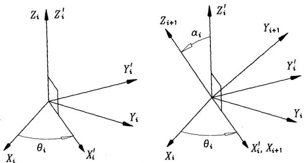
$[\mathbf{Q}_i]_i = [\mathbf{C}_i]_i [\mathbf{\Lambda}_i]_i = \begin{bmatrix} \cos \theta_i & -\lambda_i \sin \theta_i & \mu_i \sin \theta_i \\ \sin \theta_i & \lambda_i \cos \theta_i & -\mu_i \cos \theta_i \\ 0 & \mu_i & \lambda_i \end{bmatrix}$
