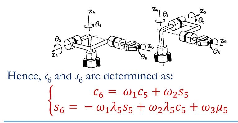
When combined with the four postures of a decoupled manipulator leading to one and the same location of its wrist center— positioning problem — a maximum of eight possible combinations of joint angles for a single pose of the end-effector of a decoupled manipulator are found
